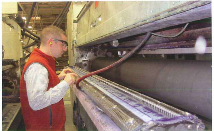
Downtime on Acme's Corrugated's Serenco jumbo flexo has been reduced, thanks to Absolute Engineering's woven carton fiber chambers, says Jeremy Cohen.
