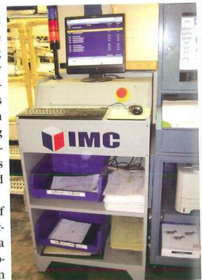
A Pacesetter control system from Intelligent Machine Control, was among the retrofits.
