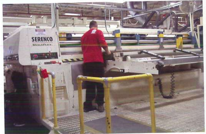
Acme's Serenco jumbo flexo, which was retrofitted with an Absolute Engineering chamber, was also repositioned in the plant to provide for an enhanced flow of finished goods.
